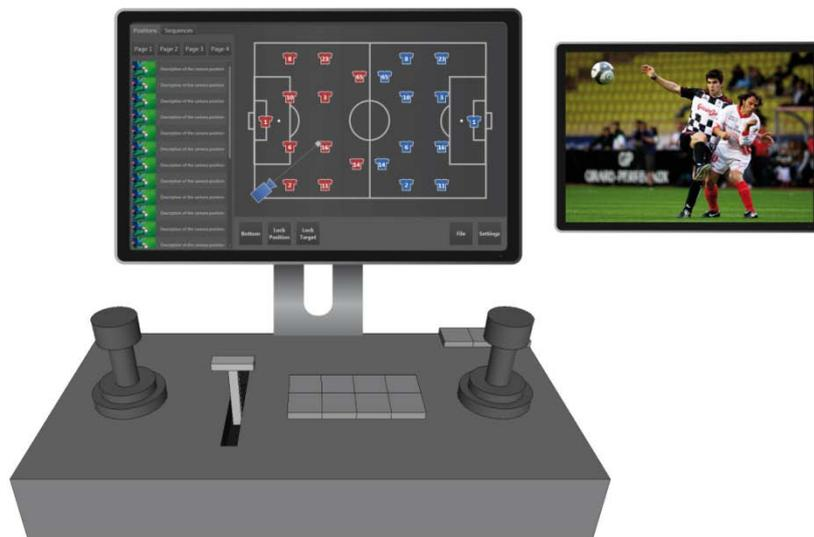
Figure 2-2 : Ideal UI for the free-viewpoint capability in the OB Van or at any broadcasting facility (Virtual Cam Console)
