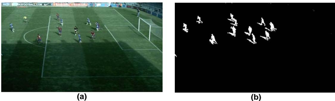
**Figure 7: Example of Background subtraction with CUDA: a) Input Image; and b) Foreground image.**
