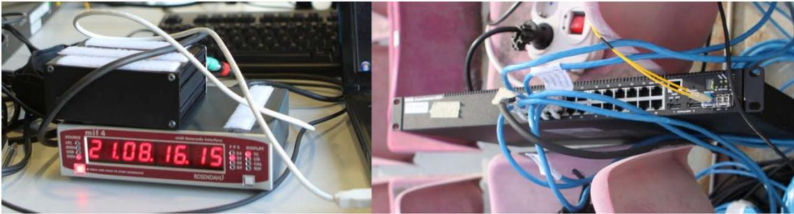
The master clock, sending pulses at 25Hz, and the main switch, transmitting the data of 8 cameras.
