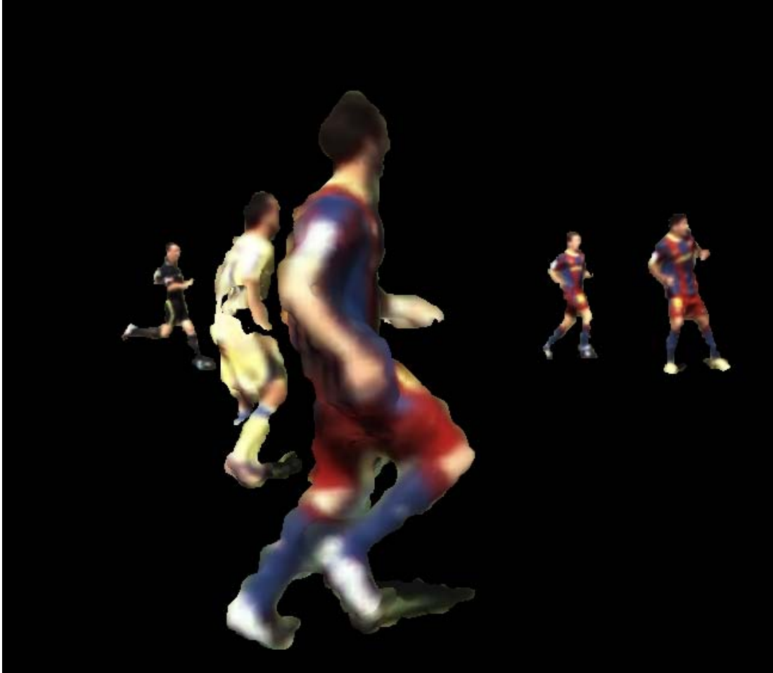
Figure 2.2: Shaded 3D mesh with colour vertex information
